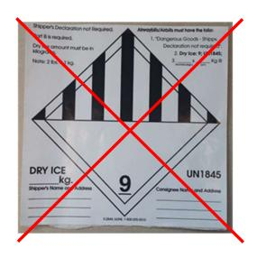
The Class 9 Miscellaneous hazard label does not contain a horizontal line connecting the vertical black bars. Be sure to use the correct label.
